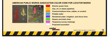
After you contact 811, the underground utility locator service will arrange for each member utility to send someone out to your dig site to mark the underground lines.
